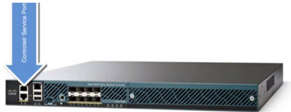
Figure 1: Service Port Location
