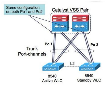
It is recommended to connect to a VSS pair and spread the links in each port-channel between the two physical switches to prevent a WLC switchover upon a failure of one of the VSS switches.
