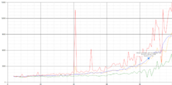
Figure 138 Sample of a VSI max response time graph, representing a normal test
