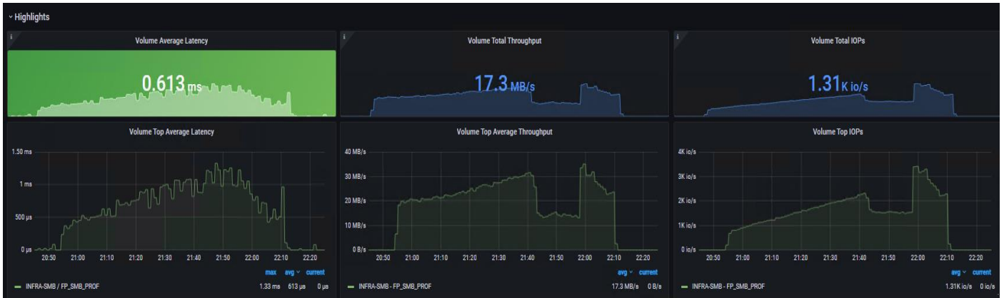
Figure 103. Volume Average Latency, Volume Total Throughput and Volume Total IOPS AFF A400 SMB Share for 1800 Full Clone Users Cluster Test
