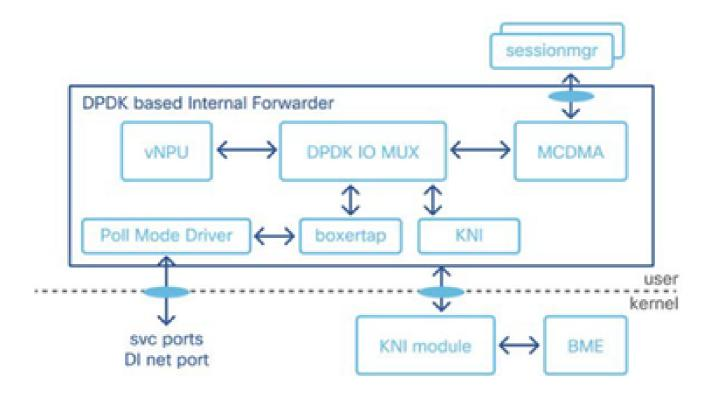
KNI: Out of Memory logs rate-limiting warnings are produced when there is a resource contention issue affecting the KNI Module.
