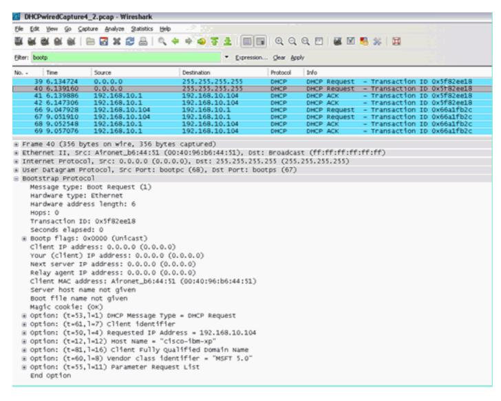
In the wired packet capture screenshot you can see that packet 40 is the bridged DHCP Request broadcast from the test client 00:40:96:b6:44:51 to the wired network.
