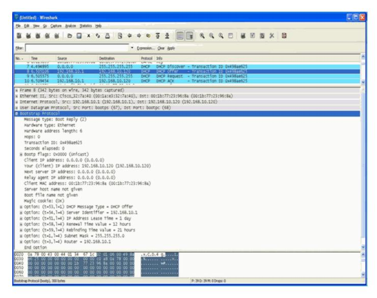
In the client-side packet capture screenshot, the main difference between the client capture in Proxy mode is the real IP of the DHCP server which is seen in the Offer and Ack packets instead of the controller virtual IP address.
