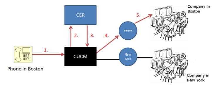
This is how a typical CER call flow works:
