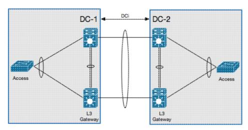
In this scenario, the Layer 3 (L3) gateway is configured on the same vPC pair and acts as the DCI. In order to isolate the HSRP, you must configure a Port Access Control List (PACL) on the DCI port-channel and disable HSRP Gratuitous Address Resolution Protocols (ARPs) (GARPs) on the Switched Virtual Interfaces (SVIs) for the VLANs that move across the DCI.
