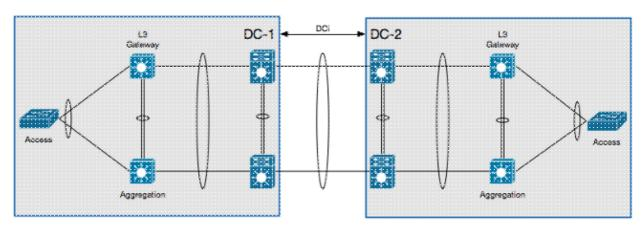
In this scenario, the DCI is isolated on its own L2 Virtual Device Context (VDC), and the L3 gateway is on an aggregation layer device. In order to isolate the HSRP, you must configure a VLAN Access Control List (VACL) that blocks the HSRP control traffic and an ARP inspection filter that blocks the HSRP GARPs on the L2 DCI VDC.
