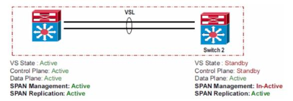
Virtual Switch System supports these SPAN capabilities per Virtual Switch domain.
