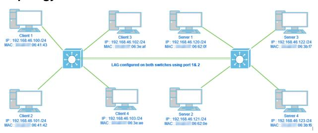
Two switches connected via LAG using 2 ports only and load balance algorithm MAC Address vs MAC/IP address. Additionally, 4 clients connected to one switch, 4 servers connected to the second switch.
