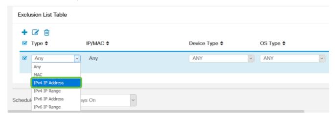
Step 18. Enter an IPv4 address in the IP field.
