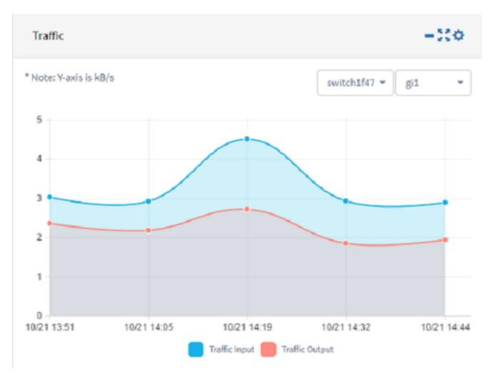
Step 1. (Optional) To hide the Traffic widget, click the **minimize widget** icon on the Traffic widget.
