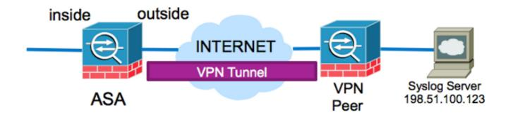
ASA# **show run logging** logging enable logging timestamp logging trap debugging logging host outside 198.51.100.123
