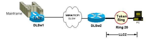
The remote DLSw+ router configuration remains unchanged. However, the LLC2 session at the central site is between the CIP and the LLC2 stack in IOS. The CIP represents the Mainframe, and the LLC2 parameters from the Mainframe out towards IOS are configured under the adapters on the LAN Token Ring (on the CIP). The LLC2 parameters from IOS towards the Mainframe are configured on the outgoing interface. That is, interface channel x/2 (for CIP) and interface channel x/0 (for xCPA). For example:
