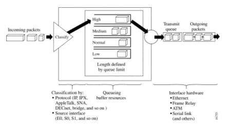
Enabling priority queueing on an interface changes the Output queue display, as illustrated below. Before priority queueing the Ethernet interface is using a single output hold queue with the default queue size of 40 packets.
