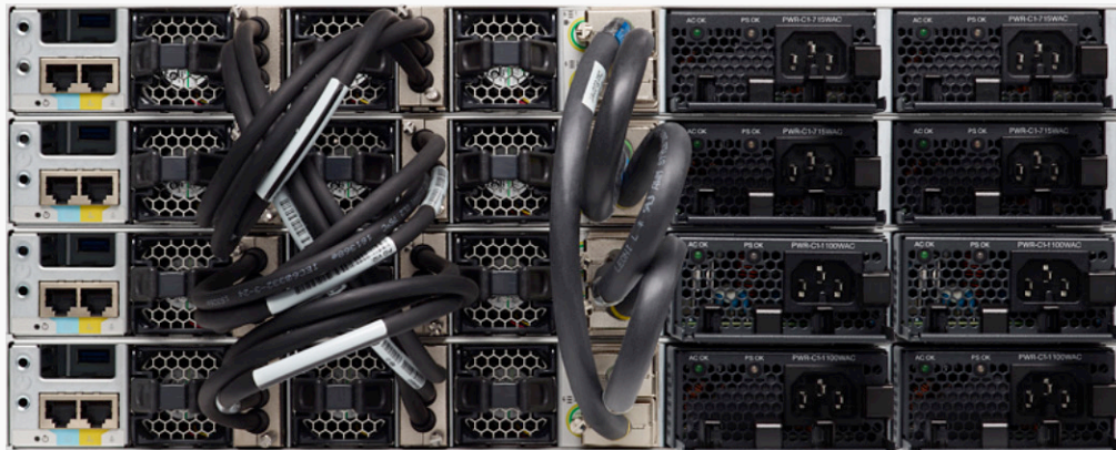
Figure 1. Cisco StackWise® 480 and Cisco StackPower connectors
