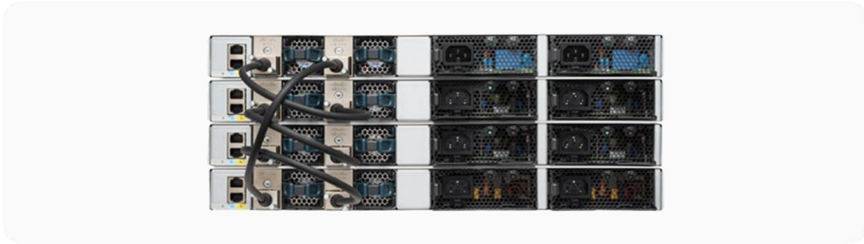
Figure 9. Switches stacked using StackWise-160
