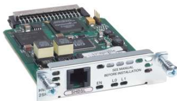
Figure 2. Cisco 4-Pair G.SHDSL HWIC (HWIC-4SHDSL)
