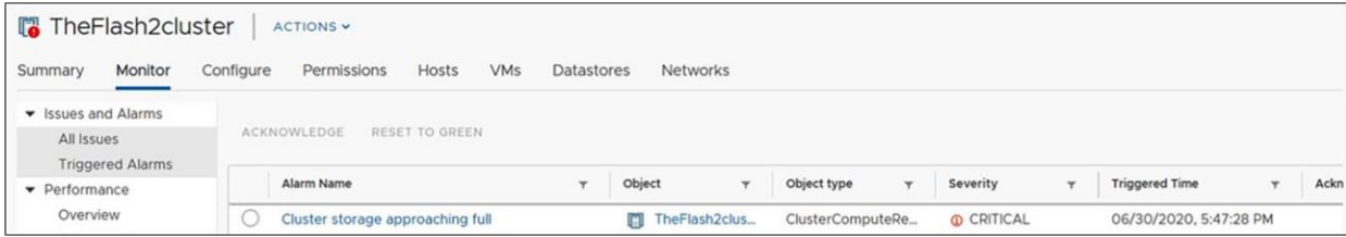
Figure 50. vCenter datastore view with severity of critical.
