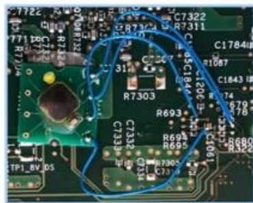
Figure 8. The Counterfeit A processor board had an "extra" component added.
