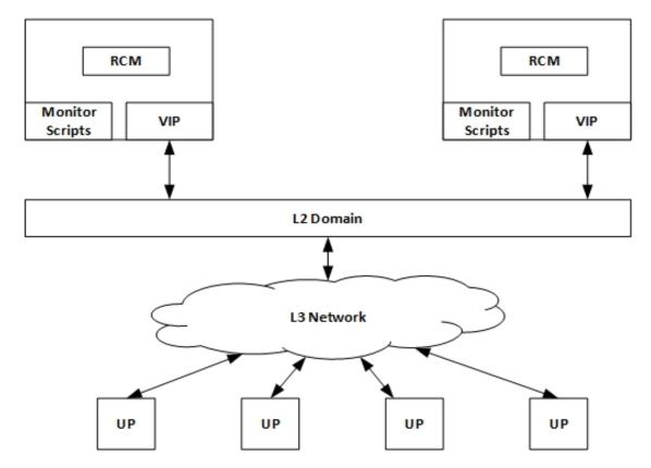
RCM HA deployments require the installation of two RCM instances instead of one. To achieve high-speed communication between the UPs and RCM, and to ensure that the UP switchover time is as minimal as possible, both RCM should be deployed in the same datacenter as the UPs for which they are providing redundancy.
