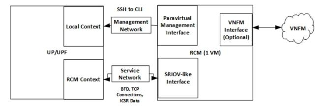
The RCM node is built on Subscriber Management Infrastructure (SMI). SMI provides the Kubernetes (K8s) infrastructure, which is used to bring all the required pods to support the redundancy for UPs.
