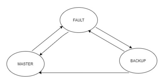
After the Keepalived pod is up and running, one of the RCM VM instances comes up as Primary and the other as Backup. When Keepalived health monitoring fails on Primary, it transitions to Fault state first and then to Backup state. At the same time, Backup transitions to Primary role. Whenever the state transitions to Fault state, the VM is rebooted. This action is done by keepalived\_notify script.
