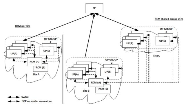
In 4G networks, UPs and CPs communicate over the Sx interface. In 5G, they communicate over N4 interface. The UP is user plane which could be a PGW-U, SGW-U, SAEGW-U, or UP(F). A group of UPs that are deployed to support the same configuration are said to be a part of same UP group (UPG). Therefore, for an N:M redundancy configuration, the UP group is comprised of (N+M) UPs that are of the same capacity and capability.
