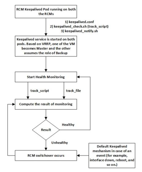
After the Keepalived pod is up and running on both the VMs, one of the RCM VMs comes up as Primary and another as Backup. Keepalived leverages the following files for proper operation:
