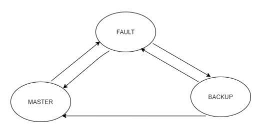
After the Keepalived pod is up and running, one of the RCM VM instances comes up as Primary and the other as Backup. When Keepalived health monitoring fails on Primary, it transitions to Fault state first and then to Backup state. At the same time, Backup transitions to Primary role. Whenever the state transitions to Fault state, the VM is rebooted. This action is done by keepalived\_notify script.
