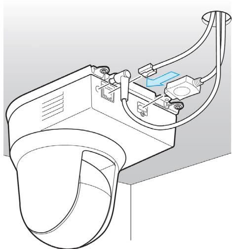
Attach the plate (1) on the back of the camera with the screw (2) and then secure the HDMI cable with a cable tie (3).
