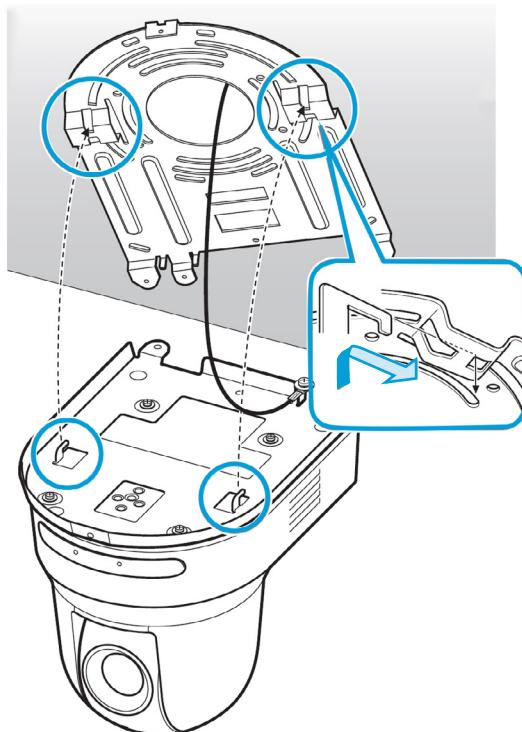
Insert the hooks on the underside of the camera into the slots on the ceiling bracket (A). Push the camera to the back.
