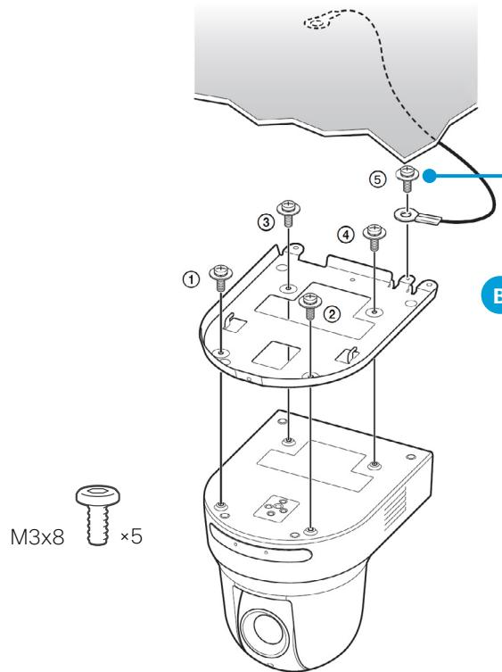
First, lightly tighten the screws in the order indicated. Then, screw each of them firmly.
