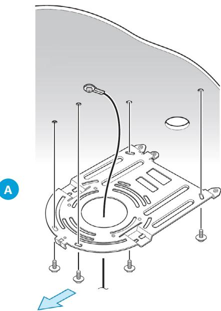
Attach the bracket (A) to the ceiling. The arrow indicates the front of the camera.
