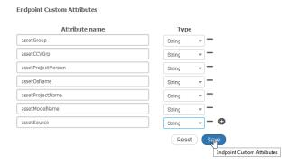
Once configured, Cisco ISE will add the value CCV in the custom attribute called assetCCVGroup if the endpoint is coming from Cisco Cyber Vision:
