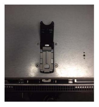
Step 8 Use the handles on the inner cover for the DIMMs to lift and remove it. A decal on the center of the inner cover shows how to safely remove it. One of the handles of the inner covers is shown below.
