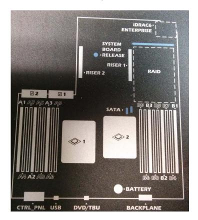
**Step 10** Remove the four 1GB DIMMs and replace them with the 2GB DIMMs, one at a time. Repeat the following procedure for each DIMM.
