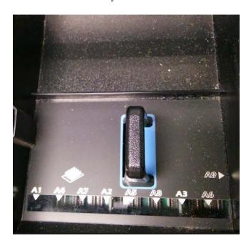
**Step 9** Locate the DIMMs in the memory slots as shown below.
