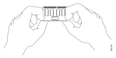
**d.** Hold the DIMM component side up, with the connector edge away from you. Line up the notch in the connector traces with the notch in the socket on the board.
