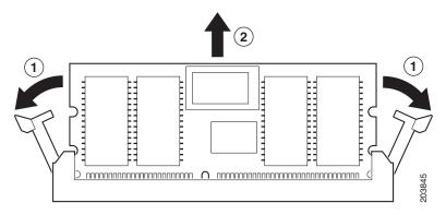
**b.** Remove the 1GB DIMM and dispose of it.
