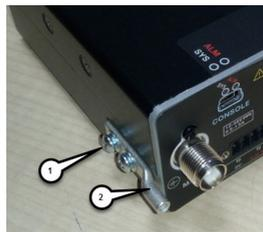
**Step 6** Use a ratcheting torque screwdriver to tighten the ground screw and ring terminal to the router side panel to 3.5 in-lb (0.4 N-m). The torque should not exceed 3.5 in-lb (0.4 N-m).
