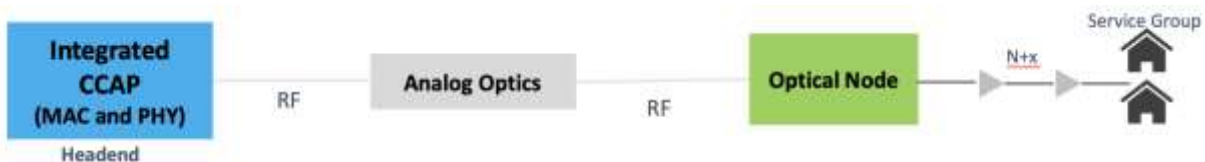
Figure 6. Legacy Network Infrastructure (simplified)
